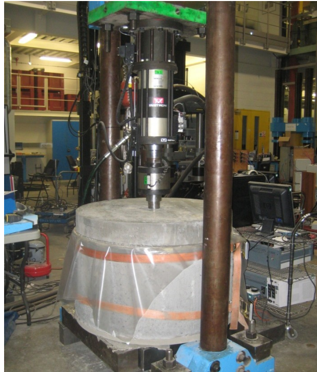
Figure 4.36: Loading arrangement of punching shear tests
