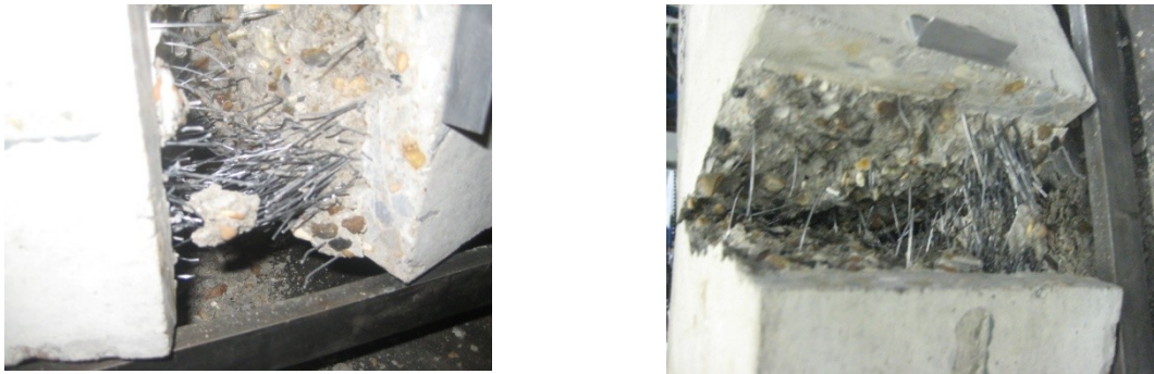
Figure 5.7: Balling of fibres in test specimen C2B6
