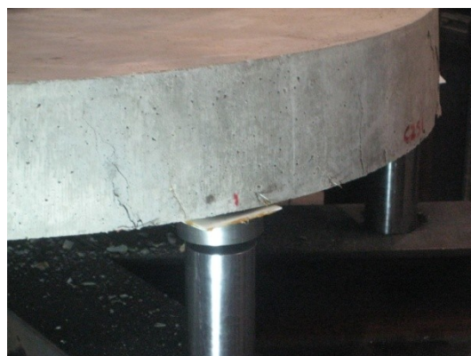
Figure 5.31: Loss of contact with support
