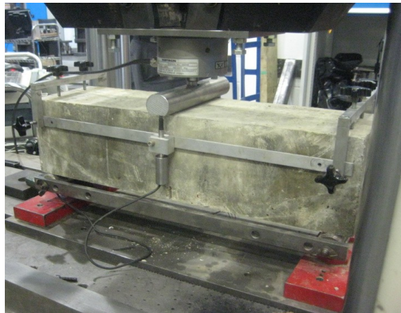
Figure 4.6: Test setup for the three-point bending beam test
