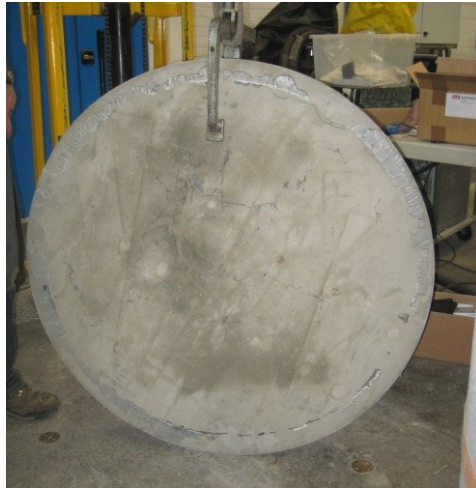
Figure 5.112: Cracking in Type II Punching Shear Tests (HE 55/25)
