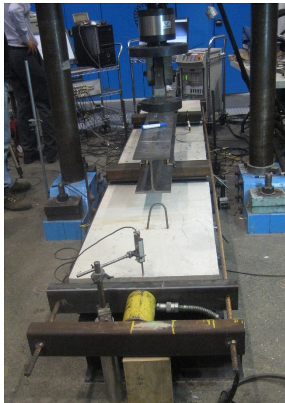
Figure 4.31: Experimental setup, using a restraint frame
