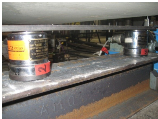
Figure 4.29: Load cells used for the measuring of load at each of the three supports
