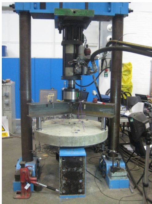
Figure 4.20: Actuator used for the present experiment
