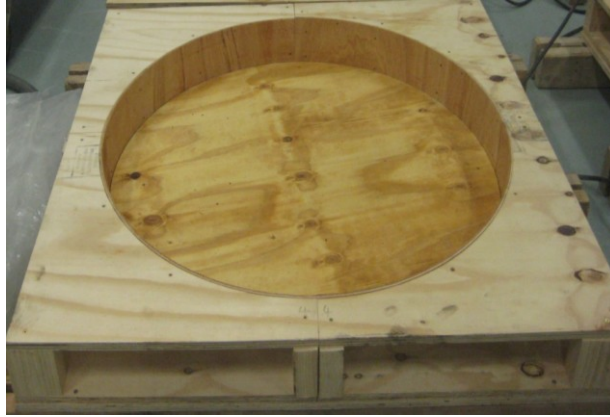
Figure 4.2: Casting mould for the round panel specimens
