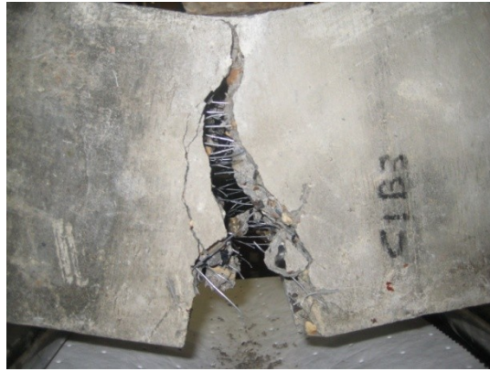
Figure 5.6: Characteristic mode of failure of a three-point bending beam test under flexure
