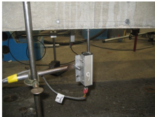
Figure 4.27: LVDT used to measure the span displacement
