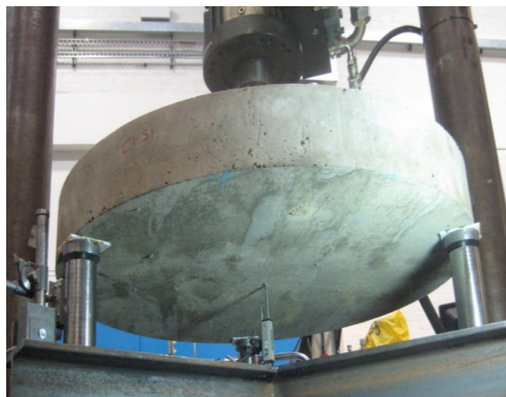
Figure 4.10: Underside of the specimen just before the commencement of the testing
