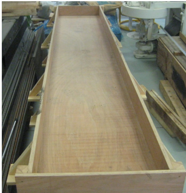
Figure 4.3: Casting mould for the long beam tests
