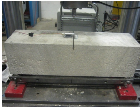
Figure 5.14: Displacement transducer for the measurement of the CMOD
