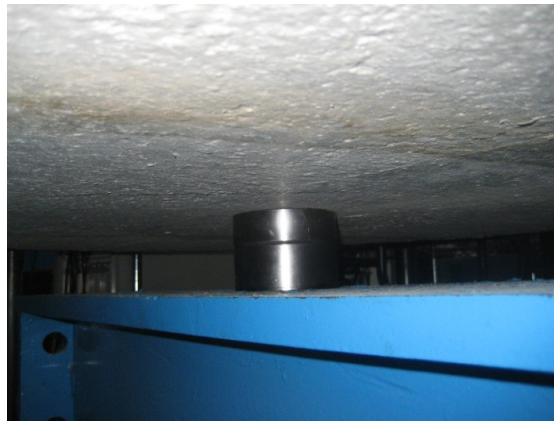
Figure 4.16: Load plate placed on the underside of the specimen
