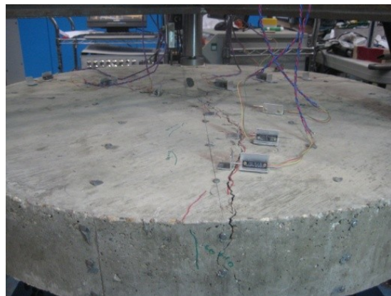
Figure 5.66: Failure Mechanism observed in slab C3S3
