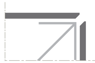
Figure 5: Mitred External Corner Detail
